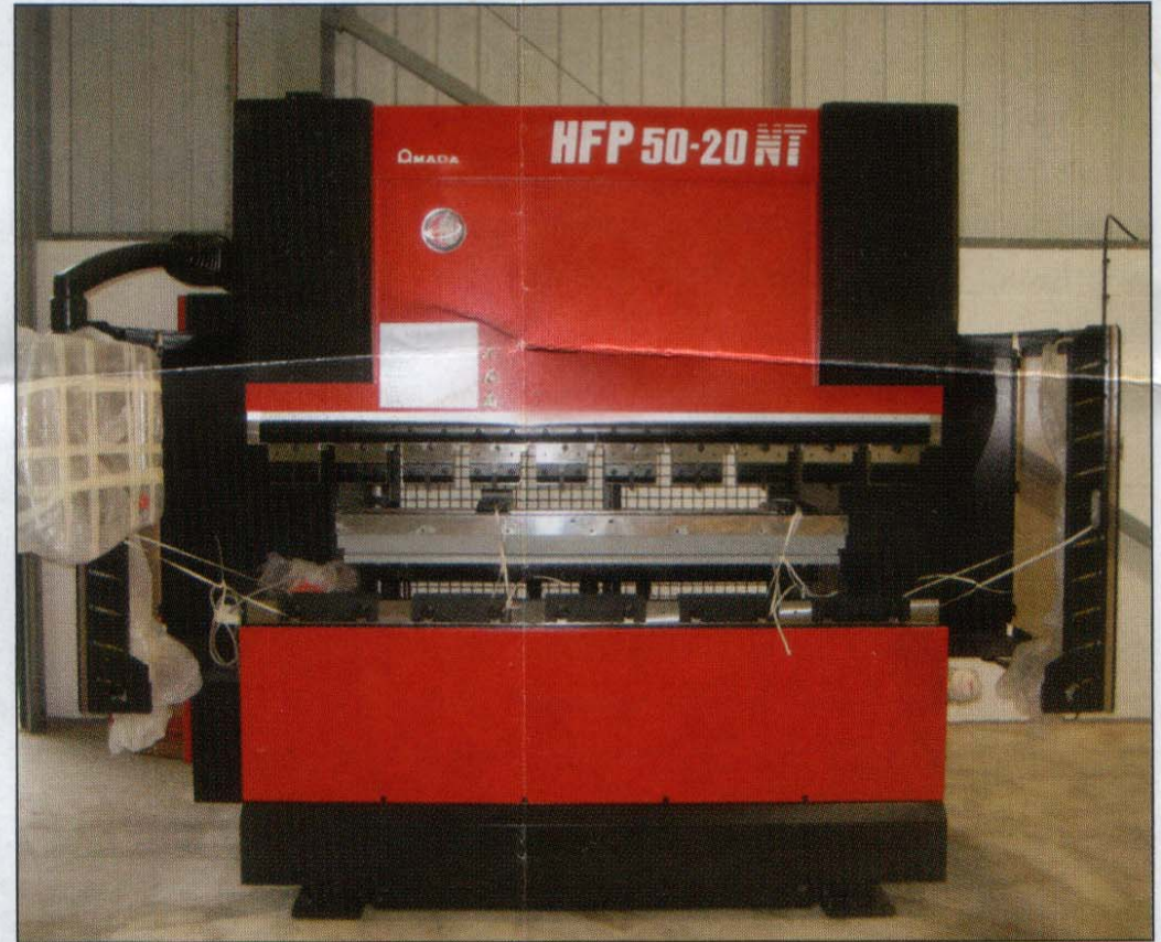
One of the two HFP 50-20 press brakes arriving at KMF's Advanced Products manufacturing facility.
